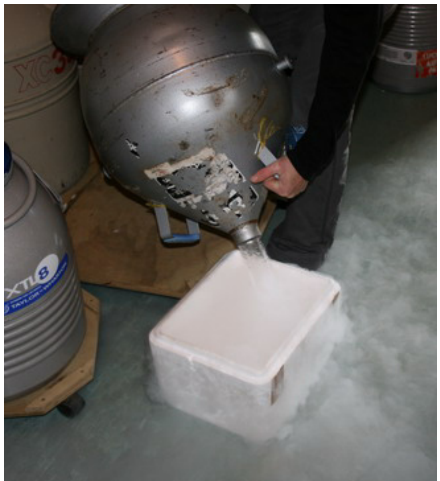
Right: Victoria pours liquid nitrogen into a temporary storage box in preparation for transferring semen to a transport container to be taken to its point of use
